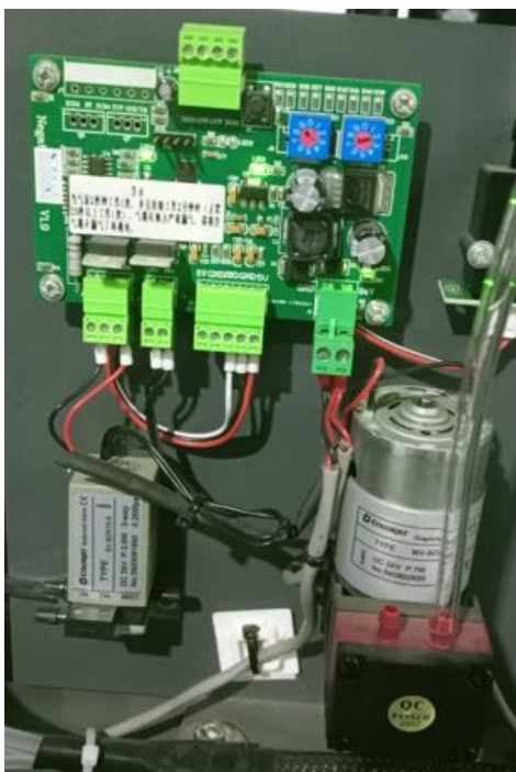
Figure 76: Negative Pressure Control Board
