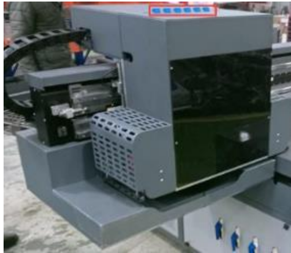
Figure 35: Closing the Sub Tanks
